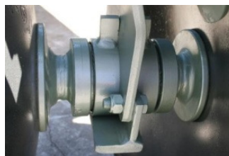
Erdvark maintenance free bearing unit.
